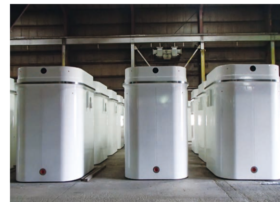
Used Fuel Dry Storage Containers fabricated by Niagara Energy Products for a Canadian customer
