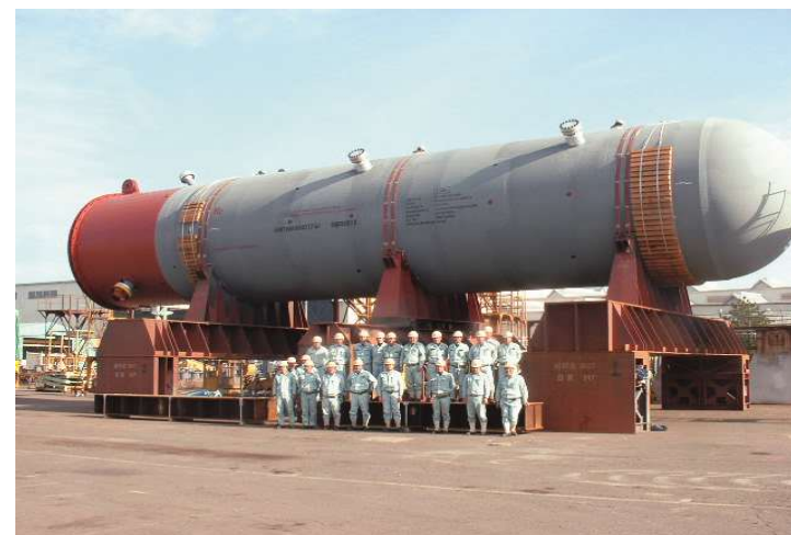
Figure A-1-15: Pressure vessel (desulphurisation reactor for Bahrain)
