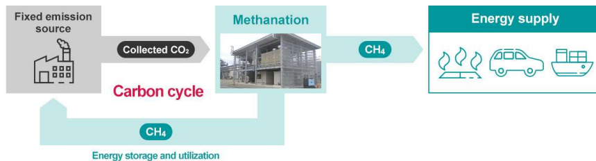
Figure A-1-18: Carbon cycle through methanation
