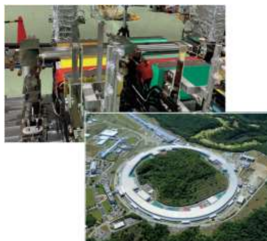
Prototype of vacuum equipment for the storage ring of the large-scale synchrotron radiation facility and a full view of the facility (Photograph of the full view of the facility courtesy of National Research and Development Agency RIKEN)
