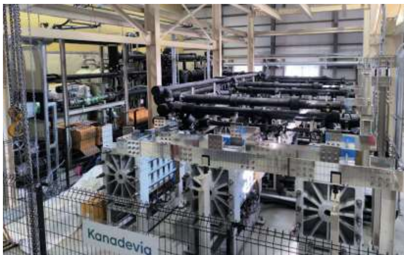
[6MW-class water electrolysis equipment introduced by the Company]
