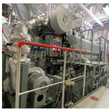
[Methane slip reduction system on board (Left: EGR* 2 system, Right: Methane oxidation catalyst layer)]
