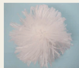
図3 繊維ろ材 (Filtration unit)
